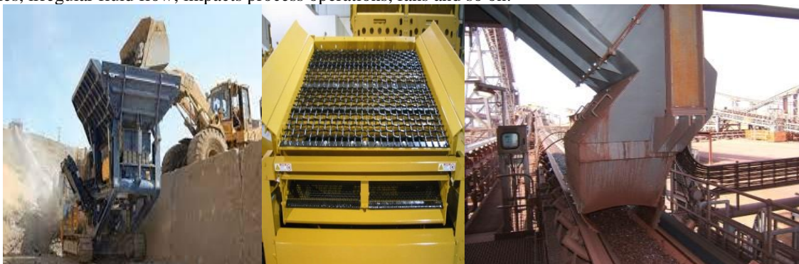
Figure 5: Crushers, Screen and Chutes (miningmagazine.com, minesep.com and im-mining.com)
