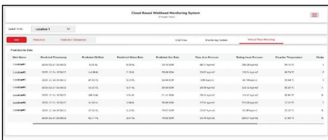
[Fig.11: Production Surveillance Dashboard on a Commercial Data Analytics Platform Showing Real-Time VFM Predictions]
